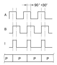
As the sensor is moved along the magnetic tape, it detects the displacement and produces an output signal equivalent to that of an incremental encoder or a linear scale.
